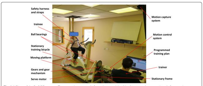
**Fig. 1** A Photo of the PerStBiRo system. The system is composed of a stationary training bicycle mounted on a moving platform, stationary frame, servo-motor, motion control system, gears and gear mechanism, two ball bearings, motion capture system, safety harness, and a trainer station (see the text for more details)
