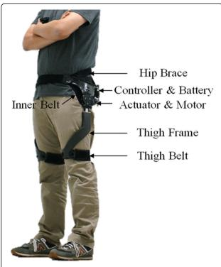
Fig. 1 Gait Enhancing Mechatronic System (GEMS)
