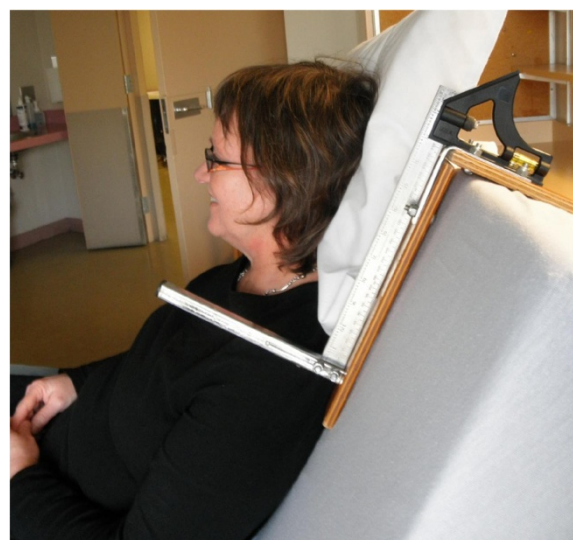
Figure 2 Trunk displacement was evaluated using a height gauge to measure the distance from the top of the mattress to the top of the shoulder.
