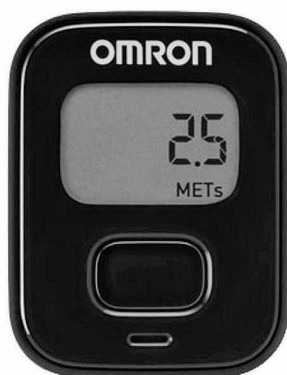
Fig. 1 Three-axial accelerometer. Active style Pro HJA-750 C (OMRON Co., Kyoto, Japan)
