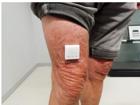
Fig. 1 A MOX device attached to the upper thigh of a person, approximately 10 cm above the knee. The MOX was attached using a special plaster
