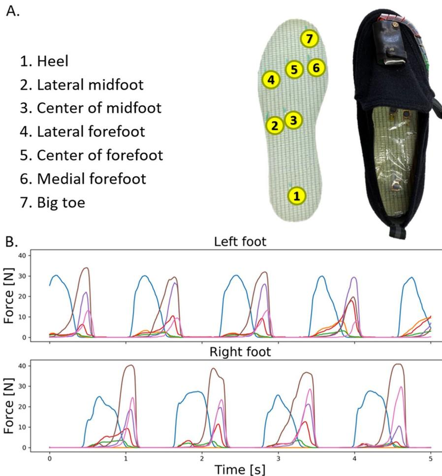
**Fig. 1** Overview of the 7-sensor plantar pressure measurement insole device and output. **A:** Seven pressure sensors are inserted in a 2 mm-thick hygienic shoe insole. The insole is inserted in a commercial Velcro shoe, and the data acquisition unit is attached using an additional piece of Velcro on the tongue. **B:** A five-second example of plantar pressure data was collected from a walking test
